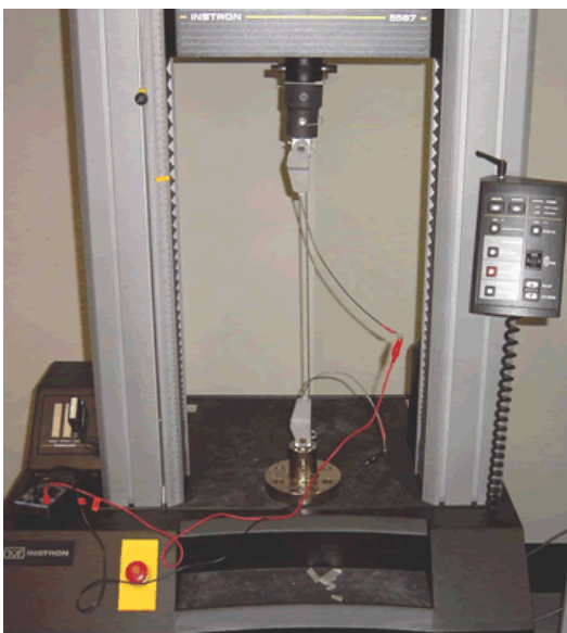
Amergraph Cable ( Under Load For Testing Purposes)
