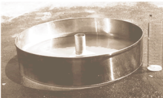
Class A Evaporation Pan complete with Fixed Point Gauge & Measuring Cylinder
