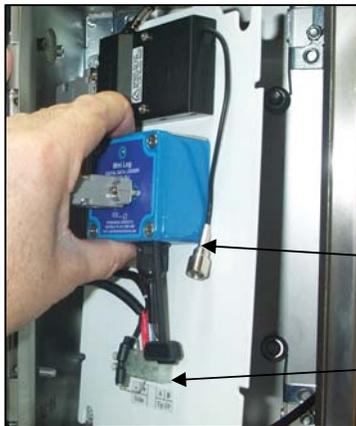
Removing electronics mounting plate
