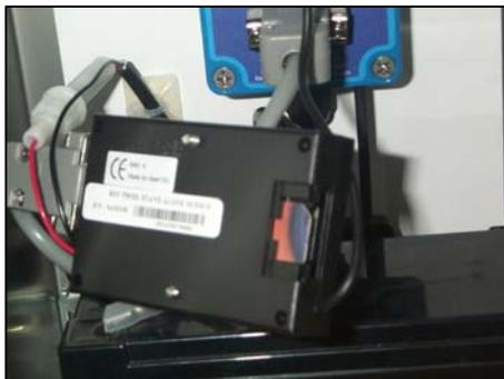
Replace the SIM card cover, and bolt the modem back onto the mounting plate.
